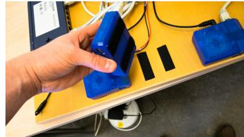
(c) Velcro-tape used to attach connected devices to the board
