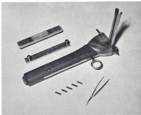
Fig. 1. Tagging apparatus. From above: tag case, tag case turned round, tagging apparatus with tag barrel (the knife is seen to the right of the ring-shaped lever), tags and forceps.
