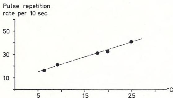
Fig. 3. Calibration line of a "thermistor tag" for plotting temperature selection of an ide.
