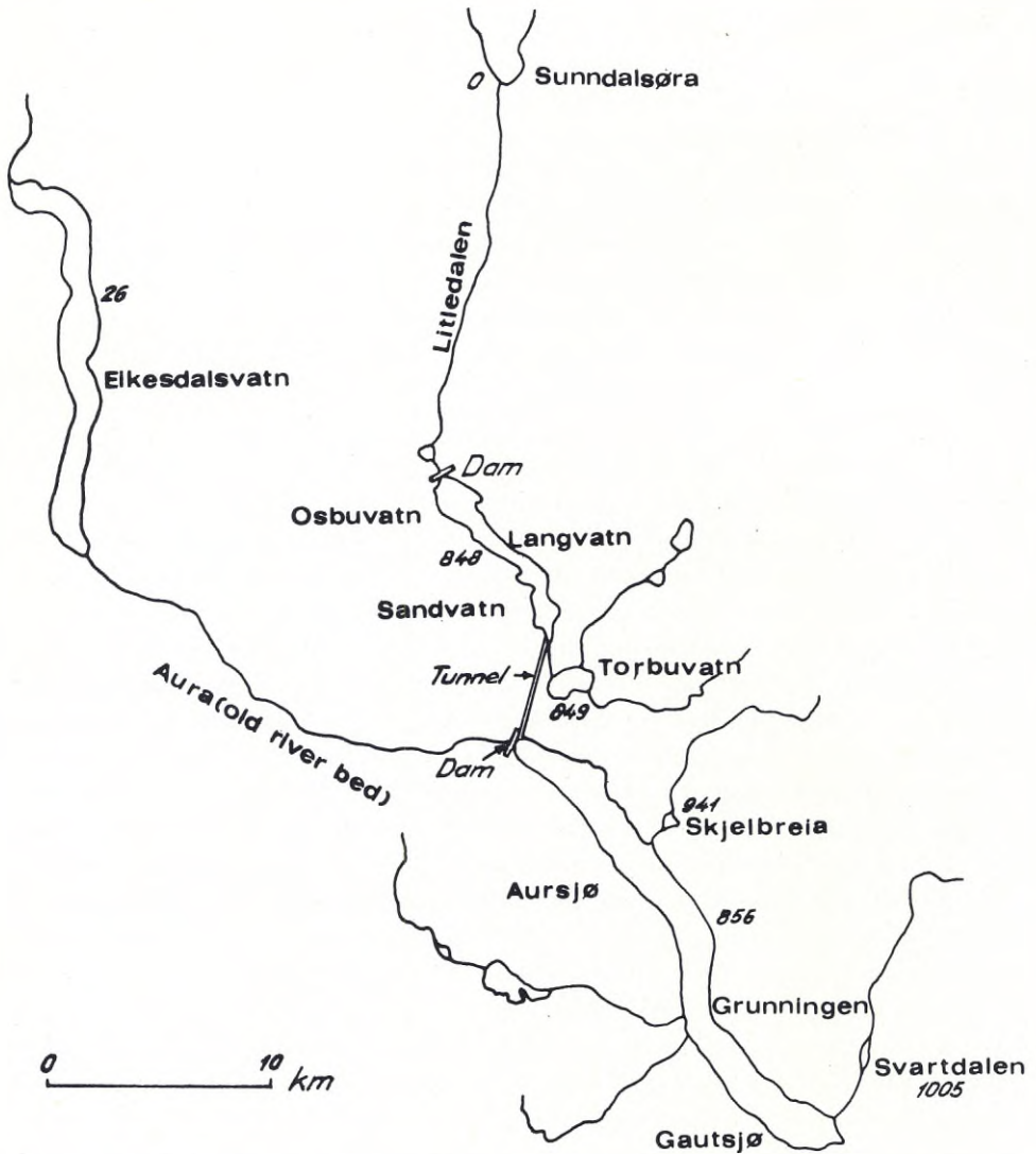
Fig. 2. Map of Aursjø and Osbu reservoirs with catchment areas. Figures indicate height in metres above sea level.
