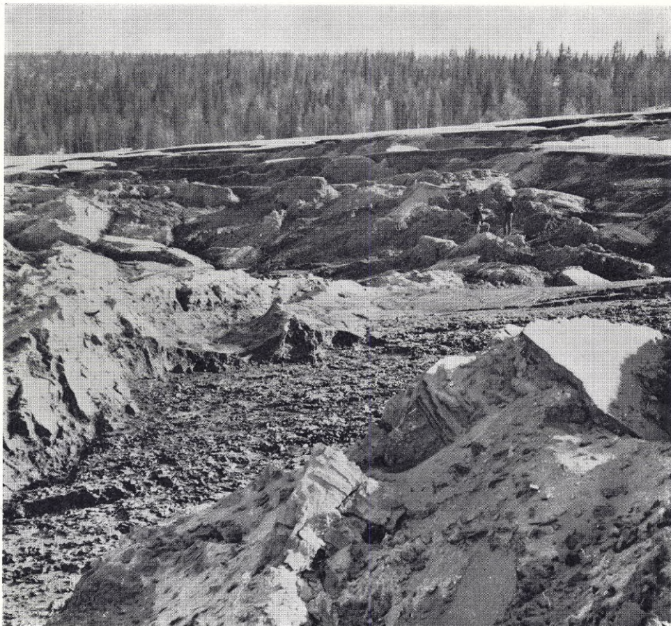
Fig. 5. Lake Blåsjön. Bottom slides provoked by the additional draw down of the water level.
