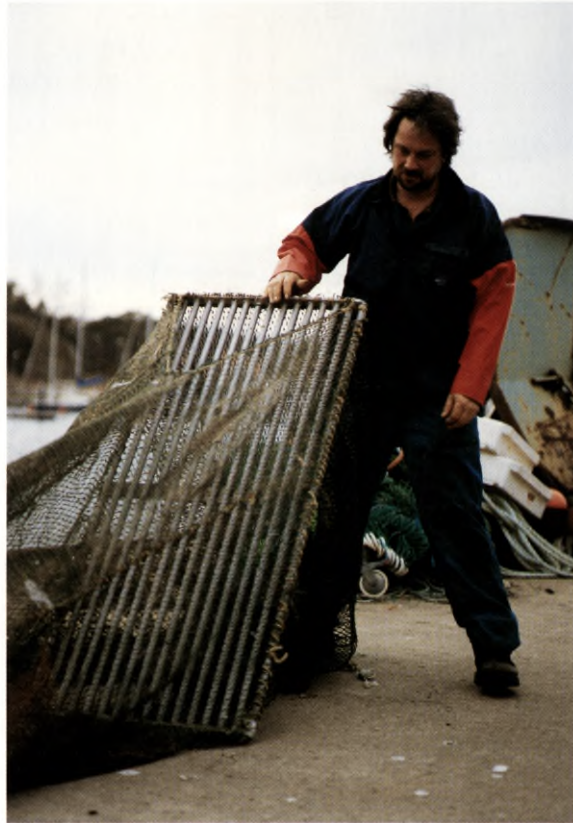
Fisherman demonstrating the Swedish Nephrops sorting grid.
