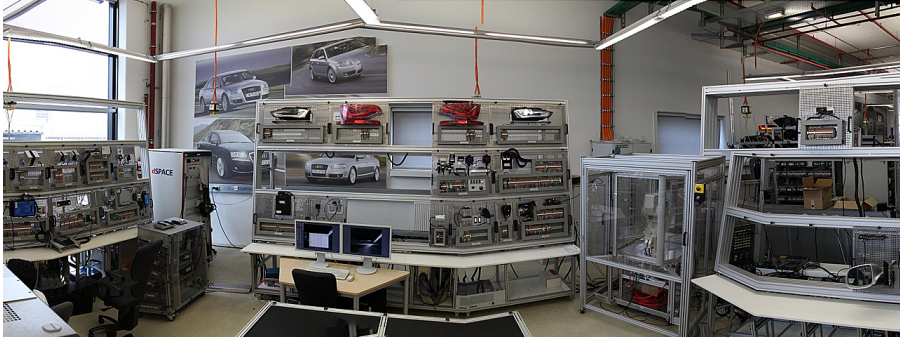
Figure 1.3: Example of a hardware-in-the-loop environment for integration testing.
