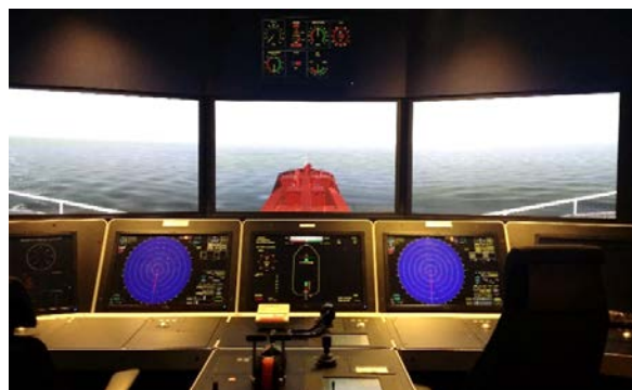
Figure 11 The Bridge Operations Simulators. This figure shows environment in which the simulation-based task or exercise takes place.
