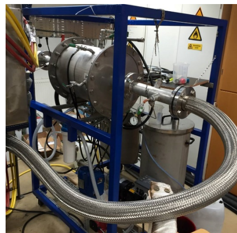
Figure 6. Schematic drawing of Chalmers' laboratory sized scrubber (left), and the actual scrubber unit (right). Water is pumped into the scrubber through six nozzles creating a mist curtain, which the exhaust gases meet when led into the scrubber. A series of perforated stainless steel plates enables efficient condensation of the wash water. Cleaned exhausts are released and scrubber water is collected or diluted. Illustration by I-M Hassellöv and photo by E Ytreberg.
