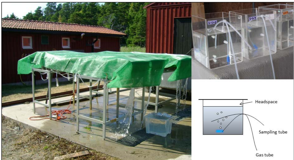
Figure 8. Experimental set-up in paper II , with green mesh covering the aquaria and continuous flow through of water (left) and the aquaria being bubbled with CO 2 -enriched air (right). Photos by M Karlberg.
