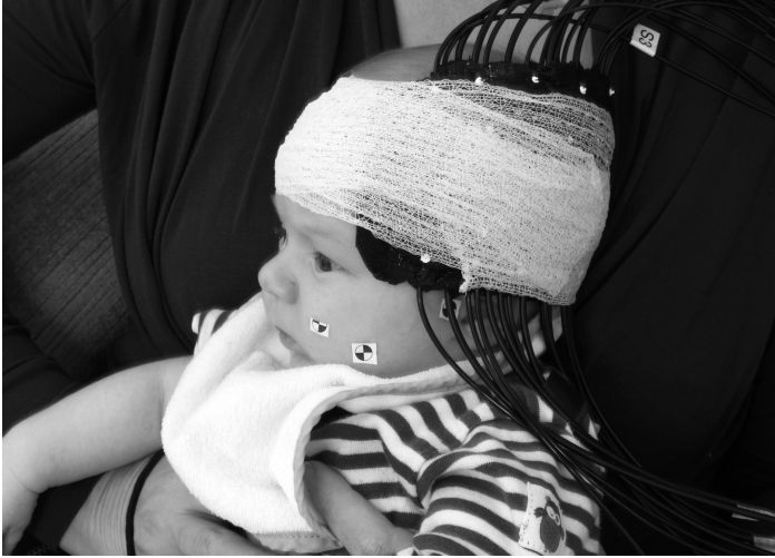
Figure 2: Experimental setup for paper I with the HD-DOT headgear attached to the head. The white dots on the probe and the black and white stickers on the skin were used to localize and coregister the obtained data.
