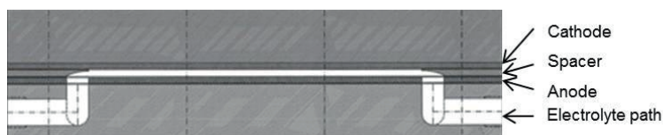
Figure 3.11 Cut through of the cells used in this work.
