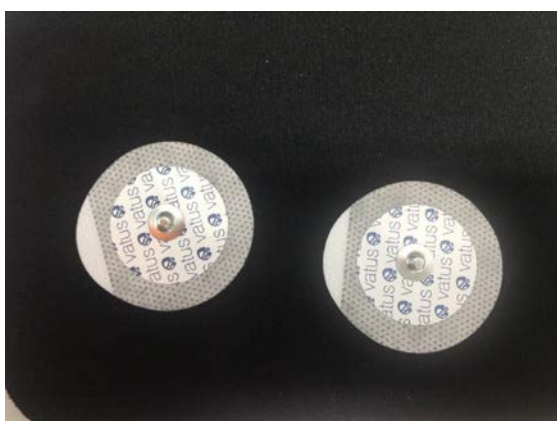
Figure 8. ECG-electrodes used as fiducial markers.
