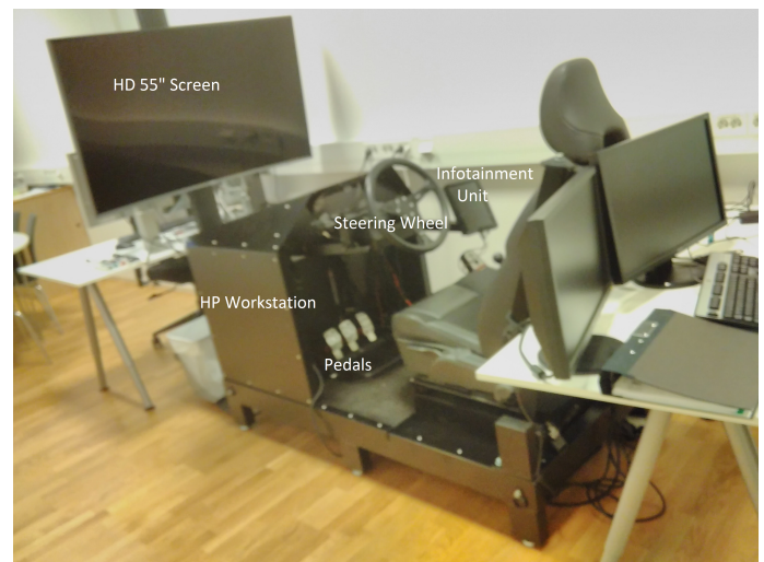
Fig. 1. HD 55" Screen, HP Workstation enclosed in the black frame, Steering Wheel, Pedals and Infotainment unit
