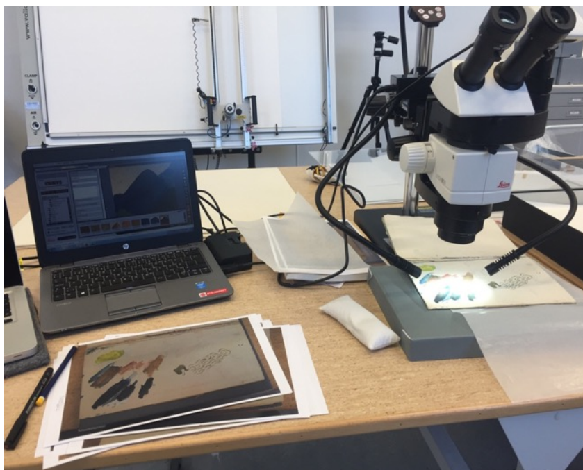
Figure 4. Microscopy setup: visual examination of the pigments in sketch book T 19/2001, with Leica M80 microscope.
