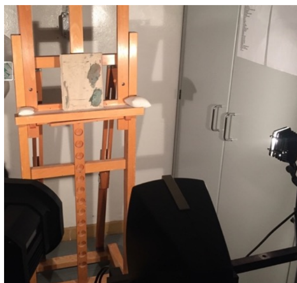
Figure 8. MSI analysis setup: collecting images of the pigment areas in various spectral bands.
