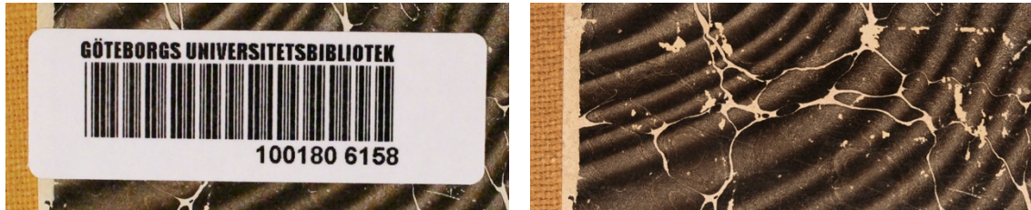
Fig. 16: 1911, vol. 32. From left to right. Before and after removal with 20% ethyl acetate solvent agar gel.
