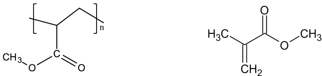
Fig. 11: From left to right: Molecular structures of poly(methyl acrylate) and methyl methacrylate (MMA). Figure created using ChemDraw Direct (Perkin Elmer 2016).
