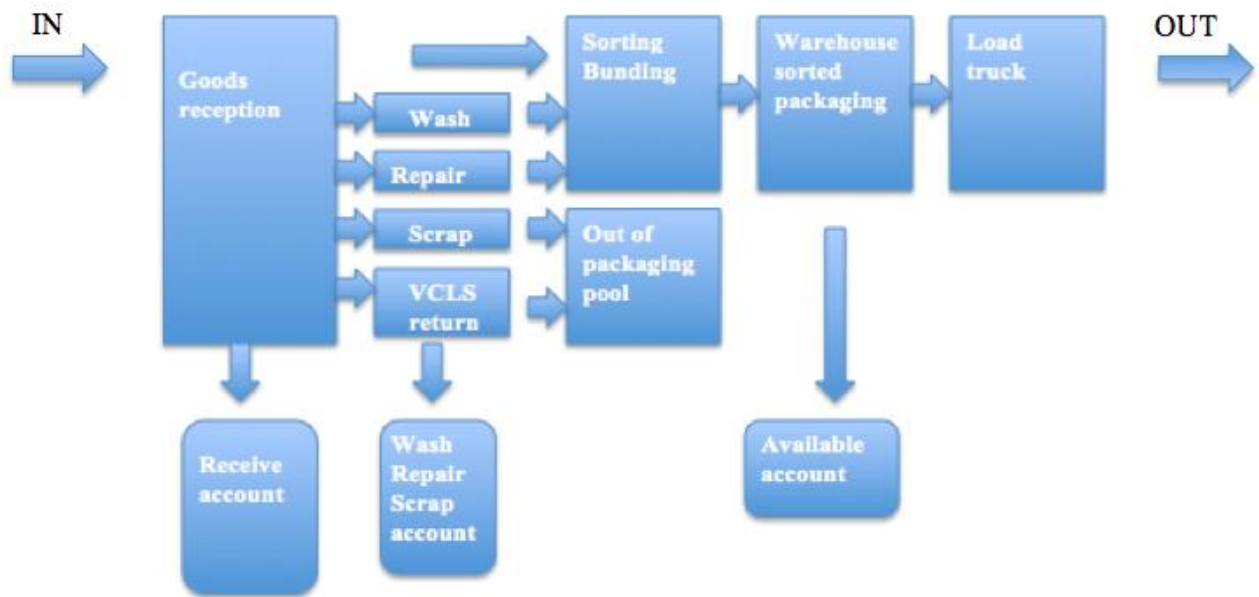
Figure 4. The Physical Flow of Packaging at Terminal. (Volvo Cars Packaging Organization, 2017)
