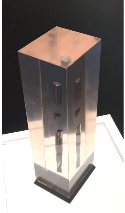
Block of resin with embed broken milling bit.
