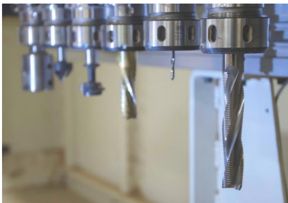
Milling drill bits
