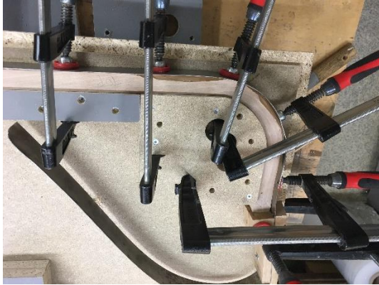
L shape steam bending in Beech wood.
