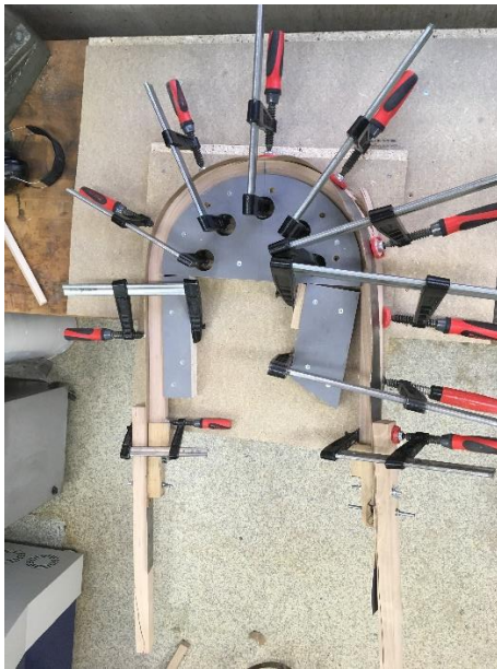
U shape steam bending in Beech wood.
