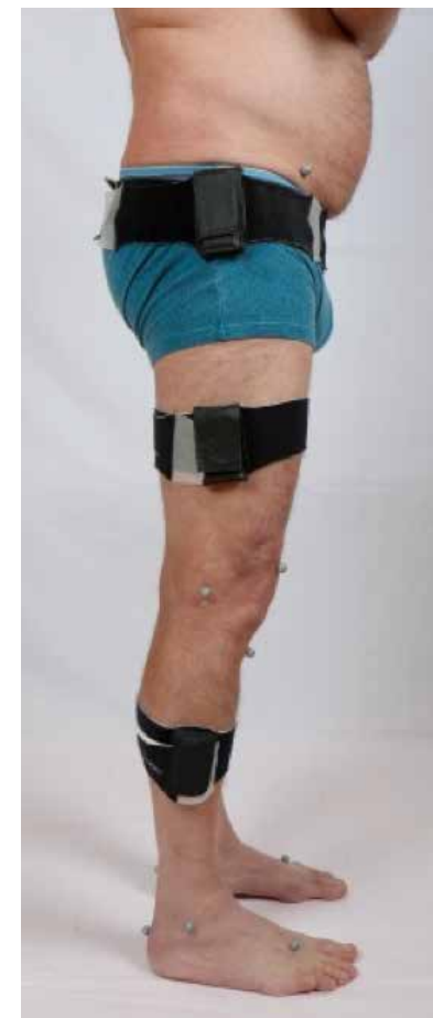
Figure 21 | Right side view IMU's together with reflective skin markers.
