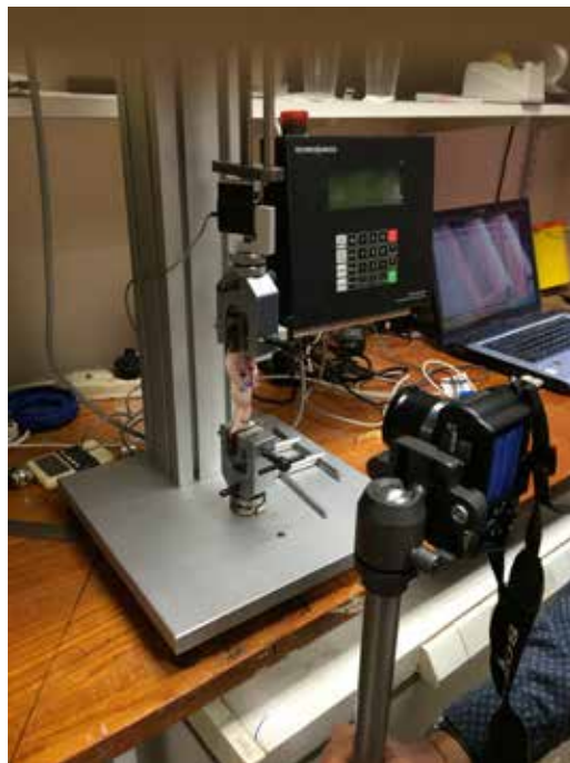
Figure 30: The tendon was clamped into a jig using sandpaper mesh and loaded using a biomechanical testing machine with computer output. A digital camera was used to record cyclical loading and testing to failure.
