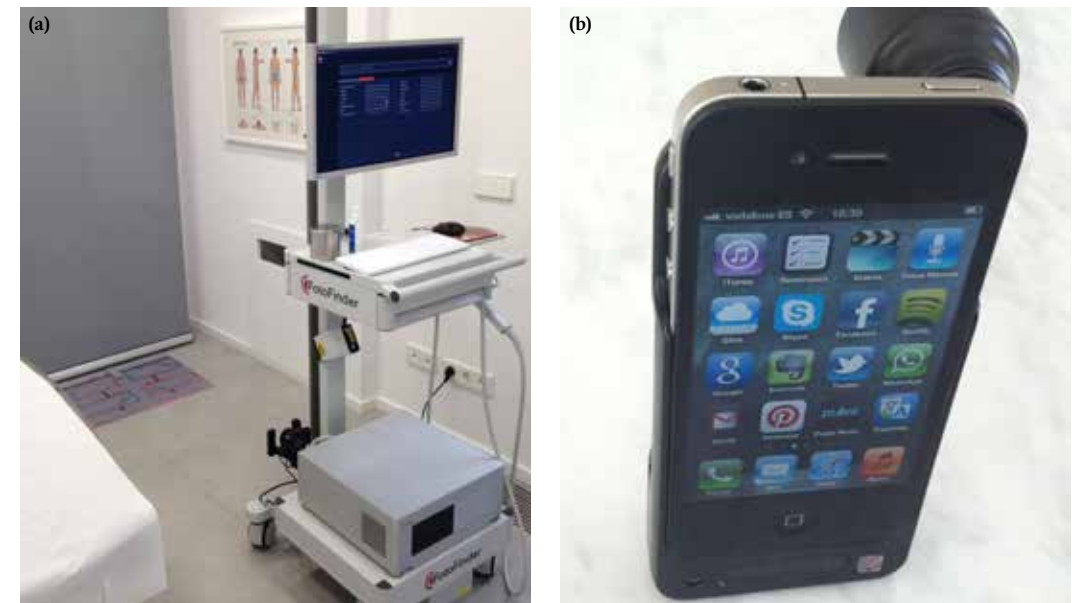
FIGURE 22. (a) A system used for total body photography (TBP) and digital dermoscopy monitoring of high risk patients. Standard positions for TBP can be seen on the wall behind the device. (b) Smartphone and dermoscope that can be used for mobile teledermoscopy.
