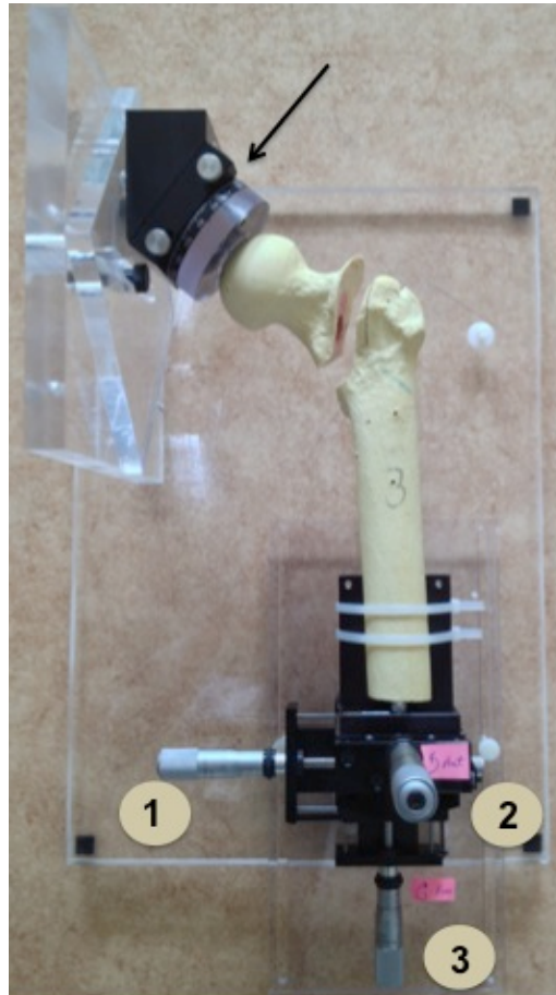
Figure 9. Phantom model of a trochanteric fracture. The knobs 1, 2, 3 of the micrometer table enable the translations in anatomical coordinate system to proximal, to medial and posterior. The femoral head, attached to a rotational table (arrow), can be rotated backwards and forwards.
