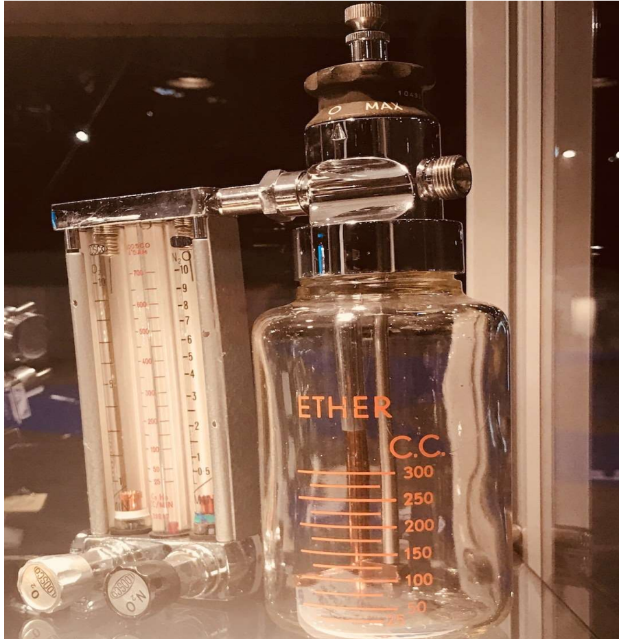
Figure 1.1 Fragment of anaesthesia circuit with rotameter and ether vaporizer from 1960. (Photo taken at medical historical display during annual ESA-meeting in Genève 2017, Sophie Lindgren)
