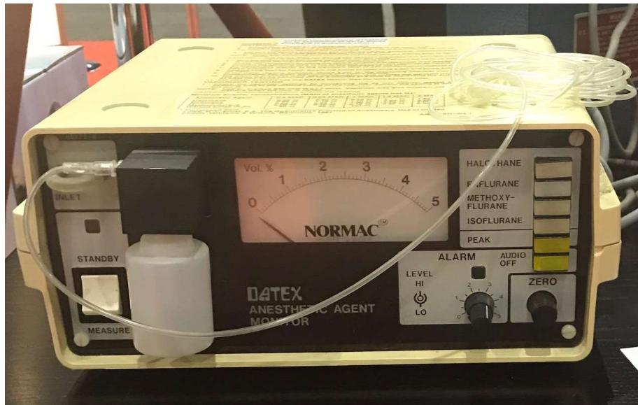
Figure 1.3 Gas monitor from the 1980s manufactured by Datex in Finland. (Photo taken at medical historical display during annual ESA-meeting in Genève 2017, Sophie Lindgren)
