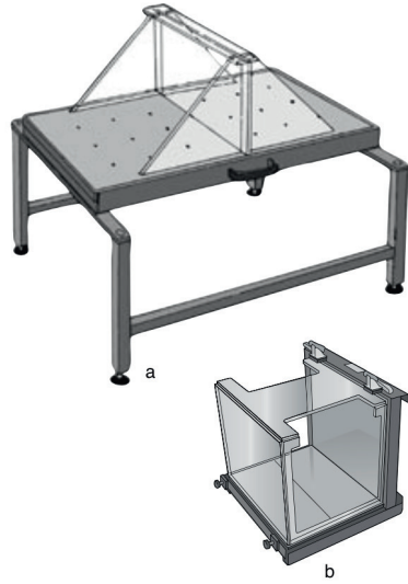
Figure 6. a) Uniplanar RSA cage, b) Biplanar RSA cage.
