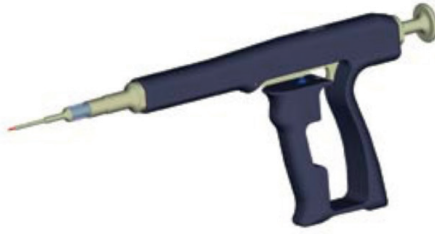
Figure 4. Illustration of the injector used for insertion of tantalum markers during a THA.
