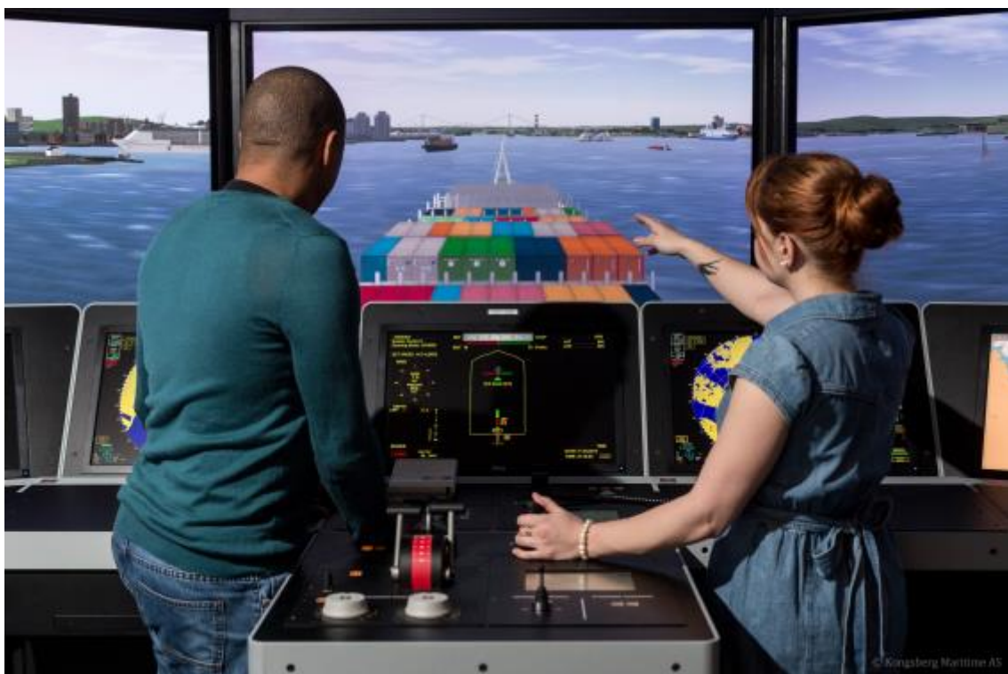
Figure 2. A bridge operation simulator equipped with systems for e-navigation. Copyright KONGSBERG Group, used with permission from KONGSBERG Group.
