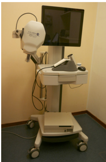
FIGURE 5. A reflectance confocal microscope at Sahlgrenska University Hospital. Photo by Morgan Carlsson.
