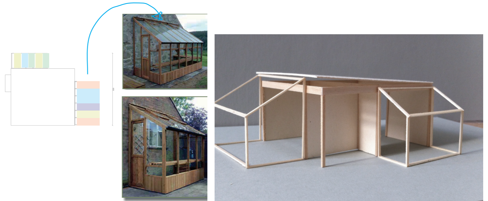
Above: Off-the-shelf potting sheds to be added to an open basic rainshed structure, offering to the dementia care home an outdoor workspace, sheltered from rain and wind.
