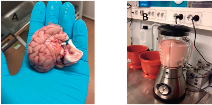
Figure 2.1: (A) Fresh porcine brains; (B) Homogenized mixture of the brains in a mixer.
