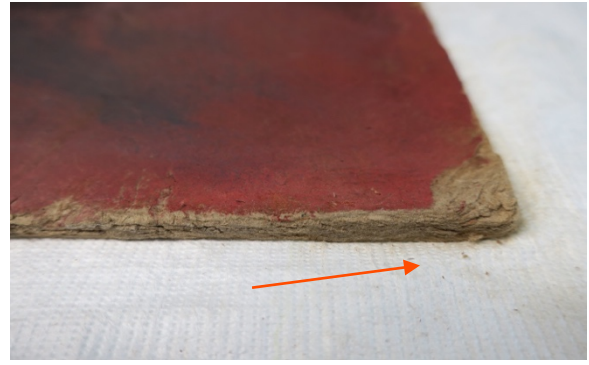
Fig. 9 Detail of the bottom right corner. The arrow indicates the detached paper particles.
