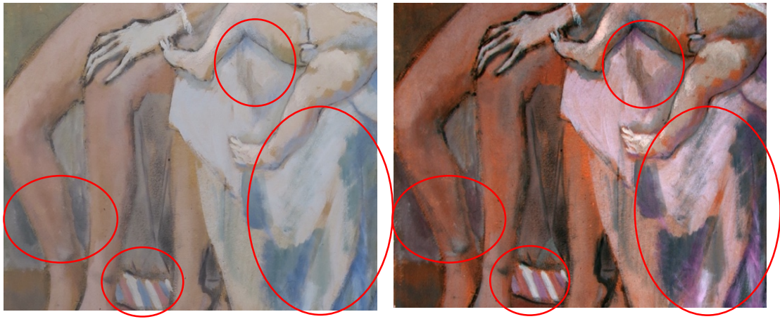
Fig. 27 MSI captures. Left: natural light. Right: infrared (band 1) false color (IRFC). The encircled areas highlight the shift of color of the blue shades when observed with IRFC, thus indicating the presence of different blue pigments.
