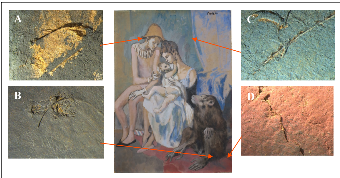
Fig. 14 Captures at 10x magnification of examples of impurities and defects. A: delamination of the cardboard. B: hair, maybe from a brush, captured in the paint. C: a feather. D: crack near the bottom right margin.
