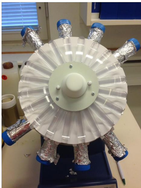
Figure 11 Samples on rotator covered with aluminum foil to avoid interaction with light.
