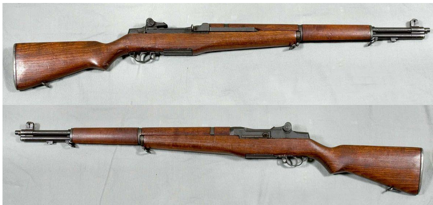
Figure 12. American made semi-automatic M1 Garand, introduced during the middle of the 1930s and one of the most famous weapons of World War 2, seen on almost every photo of American troops from the war. The weapon were unique in its design that it didn't use a magazine, but instead a clip inserted on the top of the receiver. The clip couldn't be removed without emptying it, resulting in an iconic "Ping" every time the empty clip was ejected.
