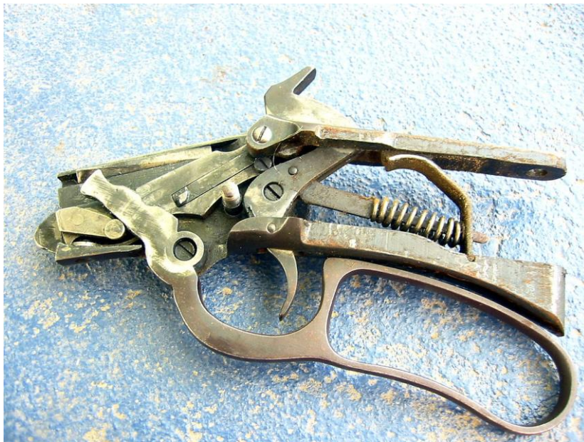
Figure 27. The inside of a Marlin 39 Lever-Action receiver. The metal has been stained because of failed removal of oil. Small traces of rust can be seen as well towards the rear end of the receiver.
