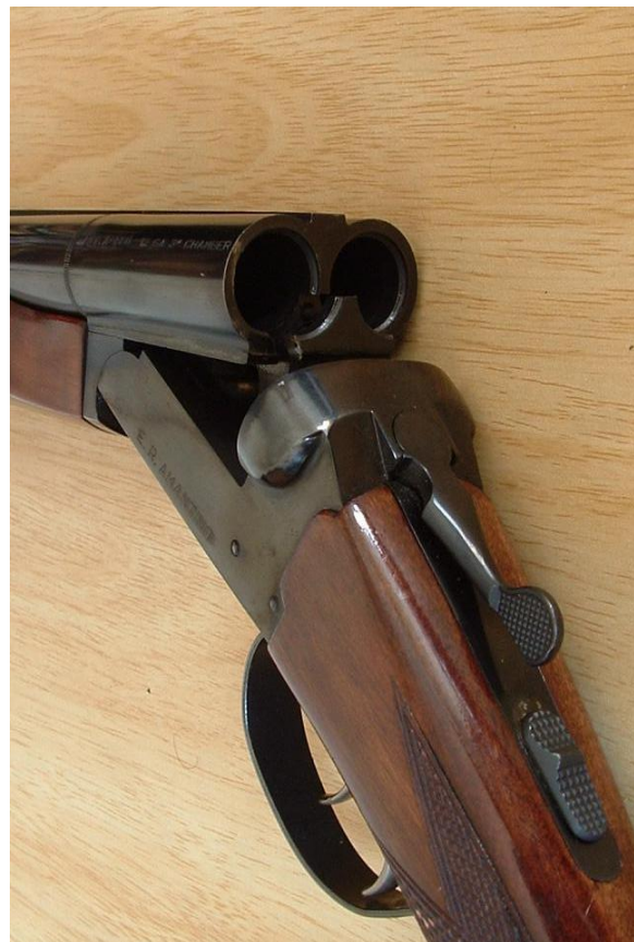
Figure 7. Common used break action function on a double barrel shotgun. The action is performed by moving the lever on top of the stock to the side.
