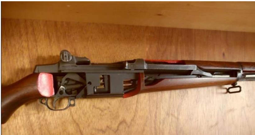
Figure 13. The inside of a M1 Garand.
