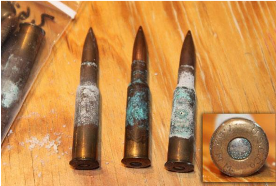
Figure 23. Brass cartridges that has been exposed to chlorides and has started to form a crust of bronze disease on top.
