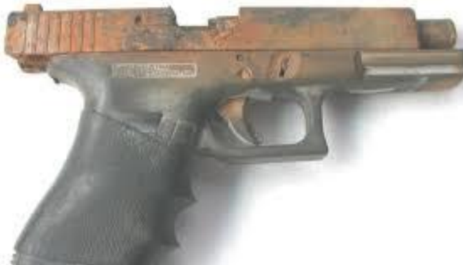
Figure 21. Rust that has been formed on a Glock 18 that has been stored in to humid conditions. The rust has stained the plastic parts of the gun as well.
