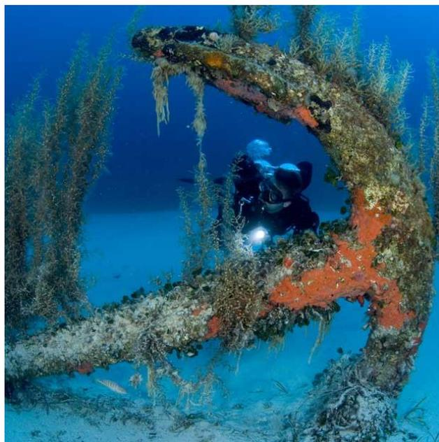
*Figure 6: Layer of marine growth upon an anchor. If it gets removed by human intervention, corrosion process might restart. (Jane Morgan, n.d.)*
