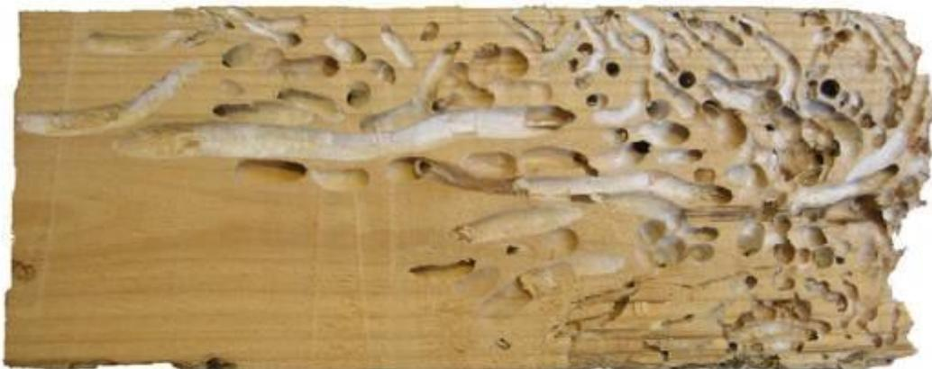
Figure 3: Degradation in the interior of wood sample caused by *Teredo Navalis*. (WreckPorotect 2011)
