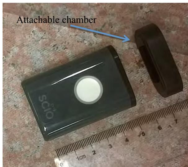
Fig 13: Size an attachable camber for SCiO. (Ingrid Sogaard 2018.)
