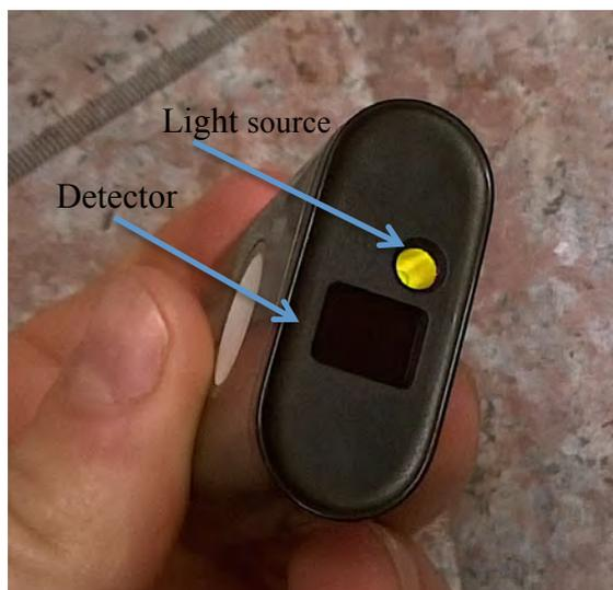
Fig 12: The position of the light source and detector on SCiO. (Ingrid Sogaard 2018.)
