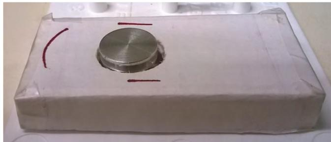
Fig 14: The scanning set-up for scanning samples on aluminium stubs. SCiO is placed on top of the sample holder. (Ingrid Søgaaard 2018.)
