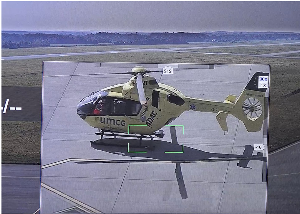
Figure 7. The Pan-Tilt-Zoom camera makes it possible to have a closer look, much like the traditional binoculars used in a control-tower (image provided by LVNL).
