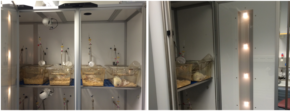
Figure 3. The Scantainer at the experimental biomedicine core facility (EBM). The rats are kept in separate cages. Cameras monitor the rats while the doors are closed. Humidity, sterile air-flow, temperature, and light cycles are standardized by the container functions.
