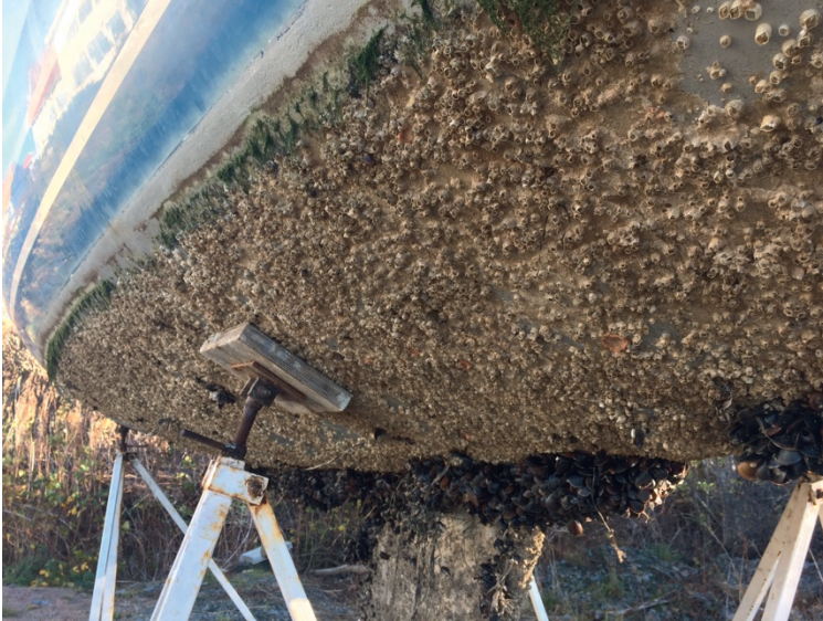
Figure 9: Picture of marine fouling on a boat hull which has not been treated with biocide-based paint (Photo: Bianca Koroschetz, 2016)
