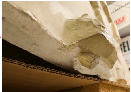
Figure 12. Two additions of gypsum are visible on the bottom of the object.
