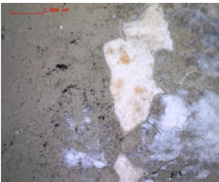
Figure 11. An area with flaking paint and gypsum or white paint on the surface. Photograph taken with USB- microscope.
