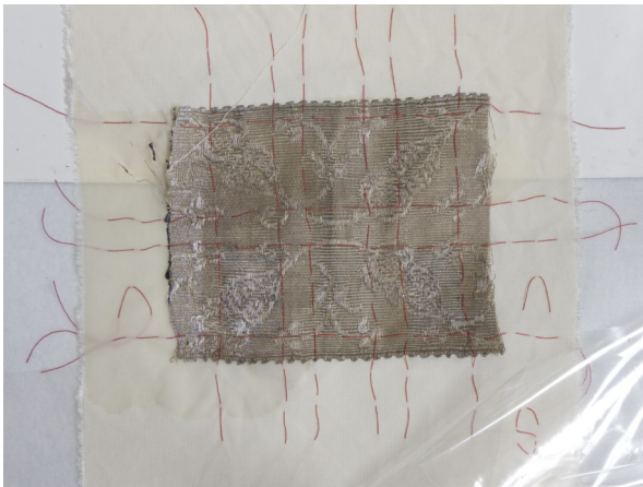
a) One of the first samples tested with the Pleco. The electrolyte has spread in the silk fabric.
