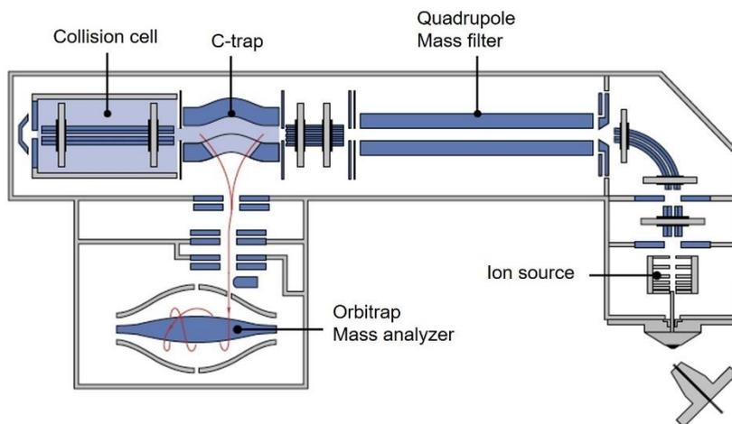
Figure 9. Schematic representation of a Q-Exactive instrument (courtesy of Thermo Fisher®)
