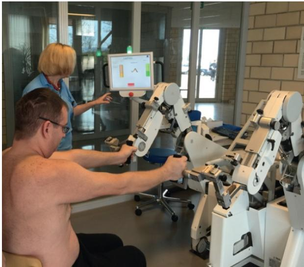
Figure 10. MotionMaker™ in the mode to measure the pushing force of the arms
