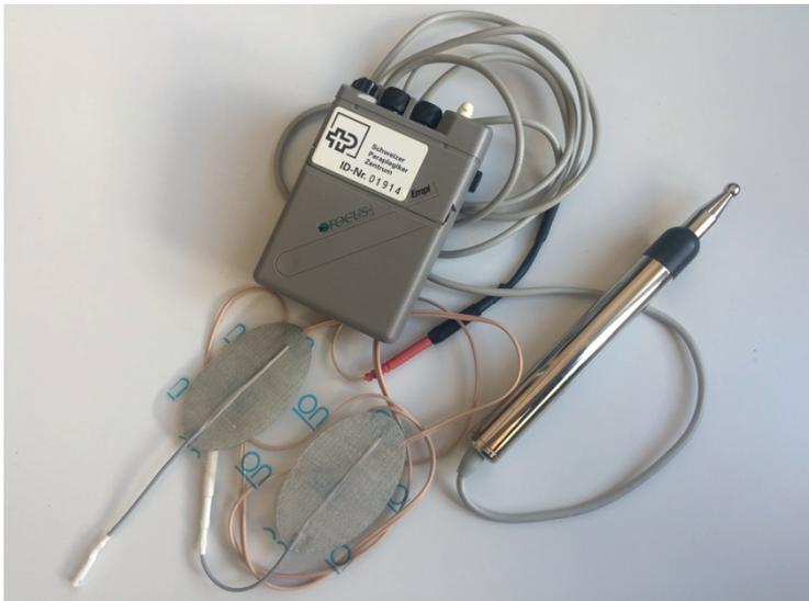
*Figure 5. EMPI 300 PV portable neuromuscular stimulator with a pen electrode*
