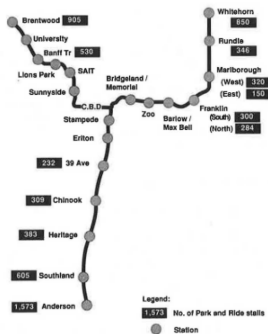
Figure 1 - LRT system and Park & Ride facilities in Calgary in 1990 (Bolger et al., 1992)
