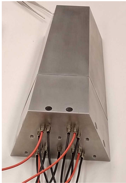
Figure 2.5: Picture of back end of Sector 1, where one can see the cables connected to the different crystals.
