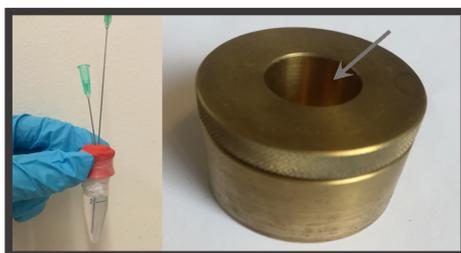
**Figure 13.** *Left:* A chopped-off falcon tube with a fitted septum that is penetrated by an inlet- and outlet needle. *Right:* An airtight cell of CaF<sub>2</sub>-glass which can be used to collect UV-Vis absorption spectra of microcrystals. The grey arrow indicates the cavity where the sample is positioned.
