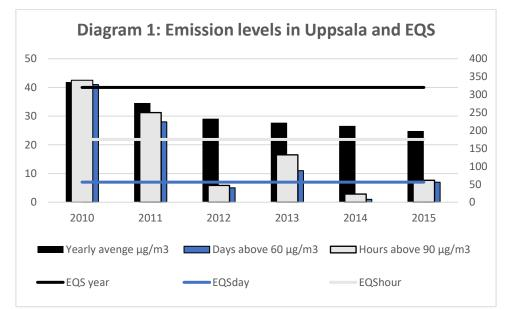
Diagram 1 shows the yearly average of NO2 levels (black bars), the number of days above  $60 \mu g/m^3$  (blue bars) and the number of hours above  $90 \mu g/m^3$  (white bars). The horizontal lines represent the EQS level,  $40 \mu g/m^3$  yearly averages (black line), 7 days (blue line) and 175 hours (white line). Observe that the black and the blue bars and lines are measured on the left axis and the white on the right. Source: SMHI (2019a)
