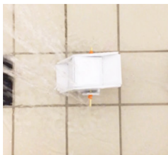
Sketch model of a rain gauge to try out the tipping function.
