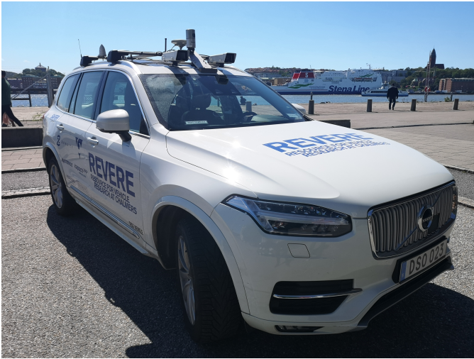
Fig. 1: Revere’s Volvo XC90 equipment with a stereo configuration of high-performance Basler cameras
