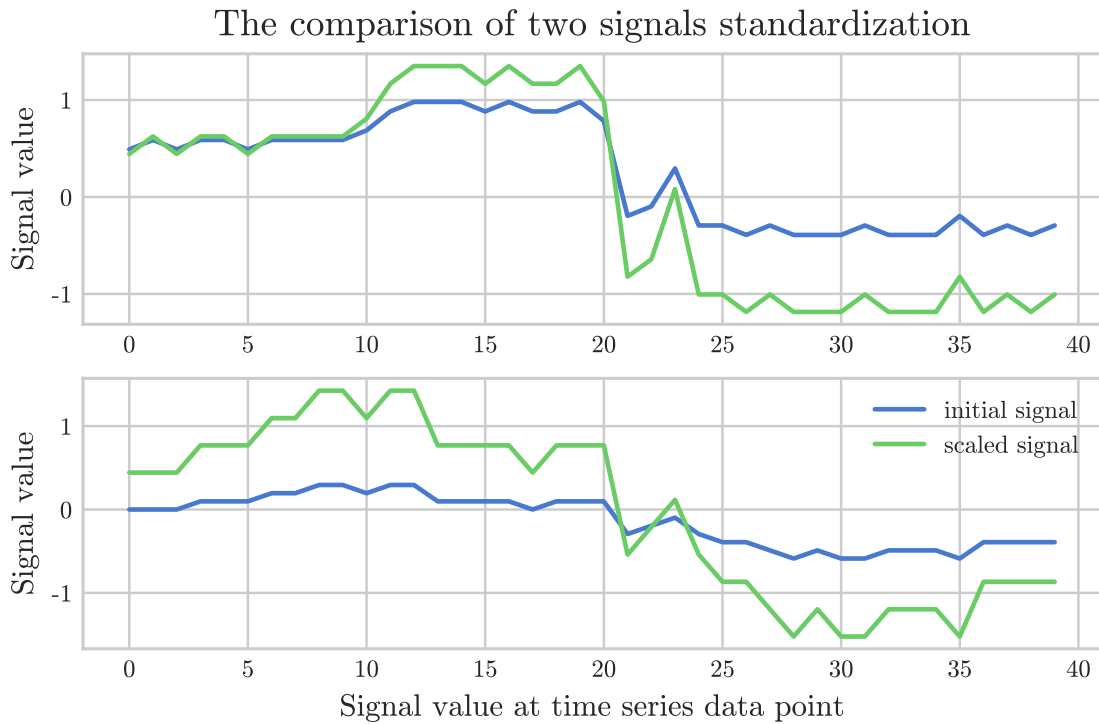
Figure 4.2: The comparison of two raw signals standardisation. Standardisation reduces the influence of a signal magnitude.
