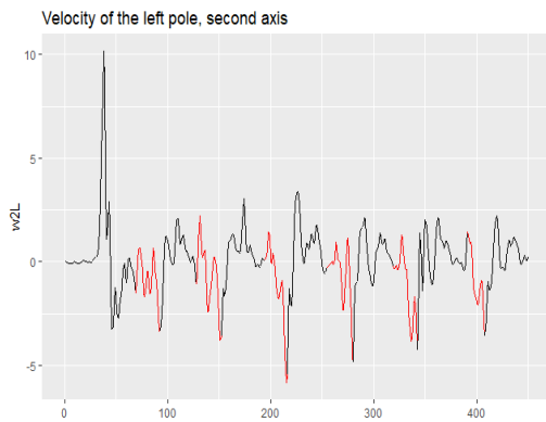
Figure 2.17: A sample of the velocity of the left pole in the second axis. The red colored parts of the curve is the time periods when there is an event in force for the left pole, i.e the skier is performing an stroking motion and generates positive force.
