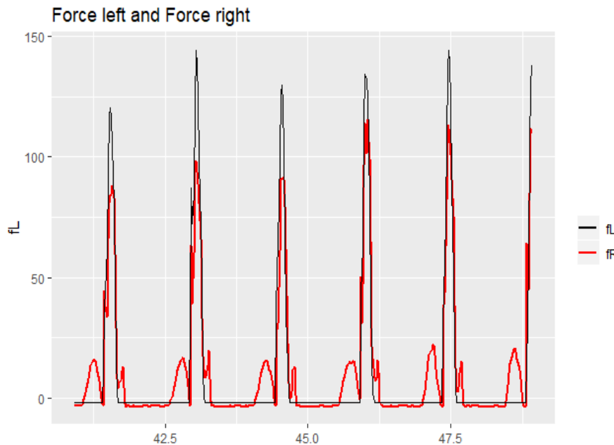
Figure 2.27: The force generated by the left hand side pole and the corresponding force from the right hand side pole during the same time period. From this small sample the existence of a systematical discrepancy in the force generated from the two poles is obvious.
