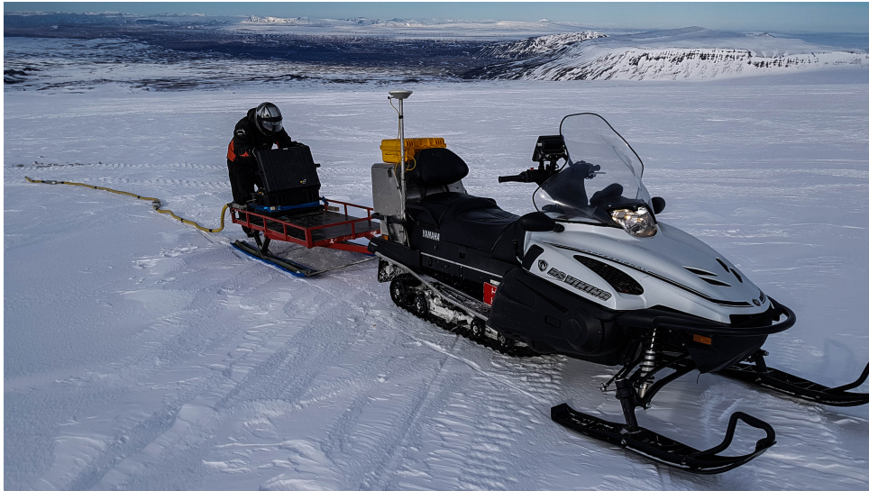
FIGURE 2.2: The GPR setup, here at Langjökull
