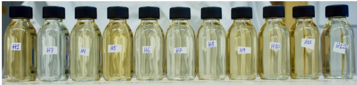
Figure 10 is a photograph of water samples from the different sampling locations in the catchment. The colour of the water correlates well to the concentration of organic carbon. The mire samples, H1, H5 and H11 are the most coloured. H3 and H12 are samples from the mineral south catchment and is almost colourless. The other samples in the photograph are all mire influenced and are all moderately coloured.
