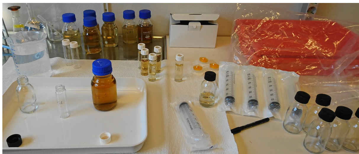
Figure 5 shows the setup when filtering the water with the water samples directly in the upper left. Vials for TOC in the middle of the picture and glass bottles for mass spectrometry on the right side.
